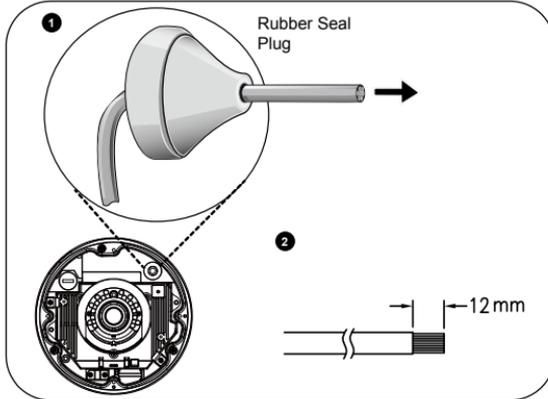
1. Drill a hole on the rubber seal plug and insert an Ethernet cable through the opening.
