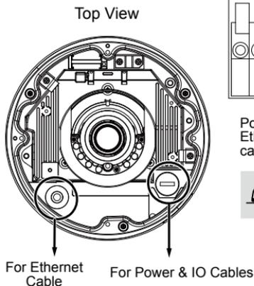
Power and IO cables pass through a waterproof connector. The Ethernet cable should be routed through a rubber seal plug. All cables are user-supplied.
