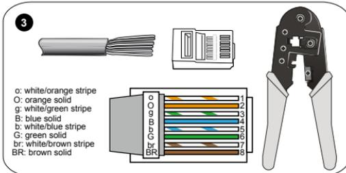
3. You will need an RJ45 crimping tool to attach the Ethernet wires to a connector. When done, connect the cable to the camera's Ethernet RJ45 socket.
