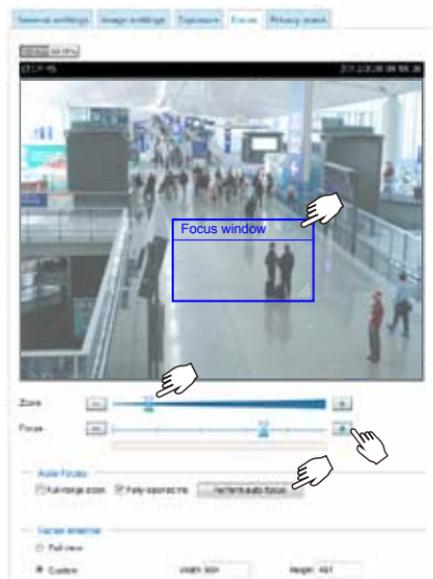
1. The camera comes with a motorized vari-focal lens module. With a web console, you can enter the **Configuration > Media > Image > Focus** page to tune the image zoom and focus.
