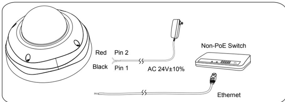
1. Connect RJ45 Ethernet cable to a switch. Use a Category 5 Cross Cable when your network camera is directly connected to PC.
